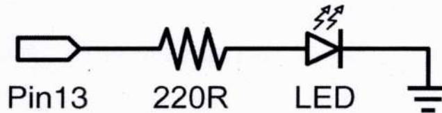
Circuit for blinking of Internal LED (No External connection required)
