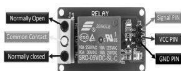
Fig 16 Relay Module Pin Diagram
